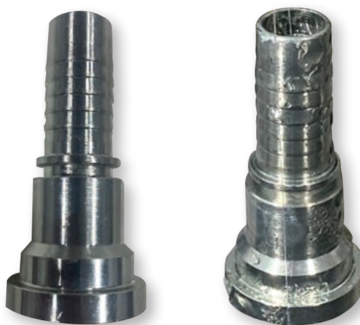
Left: Fitting prior to salt spray exposure. Right: Same fitting following 500 hours of continuous salt spray exposure.
